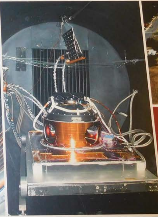
Bottom: Swift Optical Bench Thermal Vacuum Test in Facility 238
